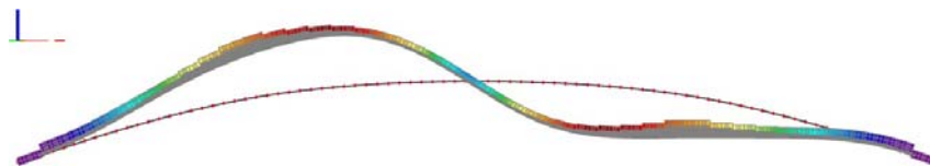
Figure 17. First vertical eigen mode
